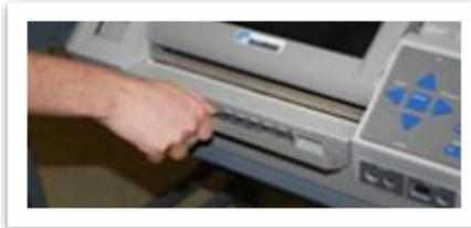
12. Power ON the AutoMARK unit by turning the gold Key to the center ON position.
